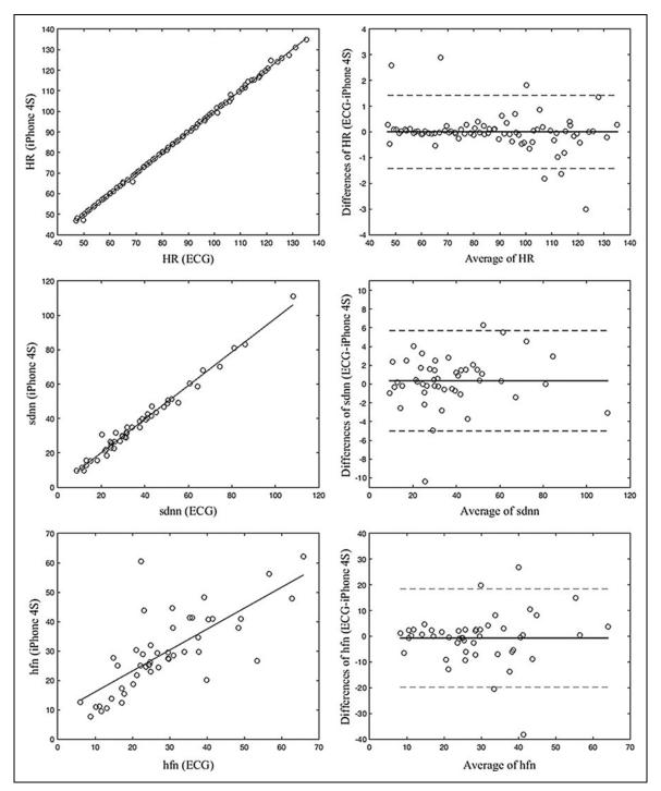
Fig. 2. Scatterplots with regression function and Bland–Altman plots of the determined HR (bpm; top) and HRV parameters sdNN (ms; center) and HFn (n.u.; bottom). HR, heart rate; HRV, heart rate variability.
