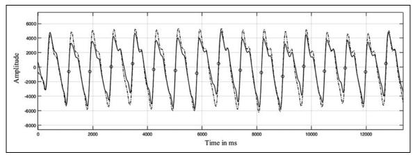
Fig. 1. Pulse curve derived from the video signal of an iPhone 4S. The circles mark the detected points in the steepest slope in each pulse wave. Original pulse wave solid line, filtered pulse wave dashed line.
